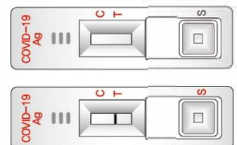
No "C" line within the result window. It is recommended that the specimen be retested.
